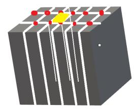
• Consider different dislocations (white) moving in a plane and cutting each other at red spots. The length between two pinning points is *L* and the height is *H*. The dislocation density in one unit cell (yellow region) can thus, be obtained as
