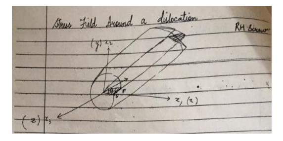
Displacement vector in x or 1 direction,  $u_1 = 0$ Displacement vector in y or 2 direction,  $u_2 = 0$ Displacement vector in z or 3 direction,  $u_3 = \frac{b\theta}{2\pi}$
