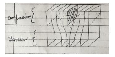
• Screw dislocation The dislocation that transforms a set of parallel planes initially perpendicular to it, into a single surface by the distortion of the planes is a screw dislocation. Differentiated into right handed and left handed, where the former is the one where b and t are antiparallel
