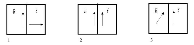
For case 1,  $\vec{b}$  is perpendicular to  $\vec{t}$  – edge dislocation For case 2,  $\vec{b}$  is parallel to  $\vec{t}$  – screw dislocation For case 3,  $\vec{b}$  is neither perpendicular to nor parallel to  $\vec{t}$  – mixed dislocation
